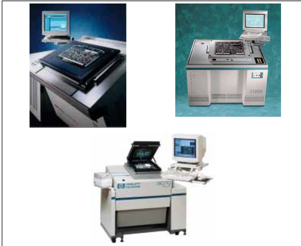
Figure 7. Automatic-Test-Equipment Programs Flash Memory On-Board
